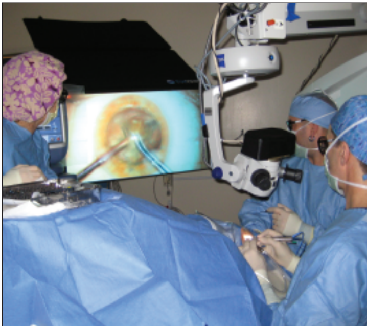
Figure 1. The 3D high-definition display screen provides imaging for cataract surgery. The surgeon, scrub nurse, and assistant wear polarized eyeglasses to resolve the dual rear-projected stereoscopic images into a single 3D image.
