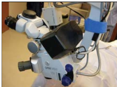
Image capture module attaches to the backside of the oculars with a beam splitting bridge.
