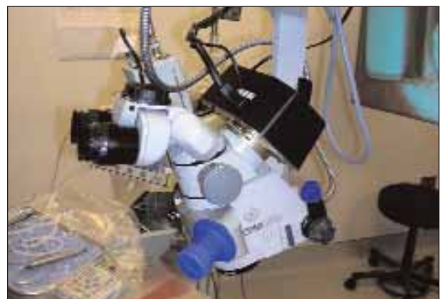
Figure 2. The image capture station sits behind the oculars of the microscope.
